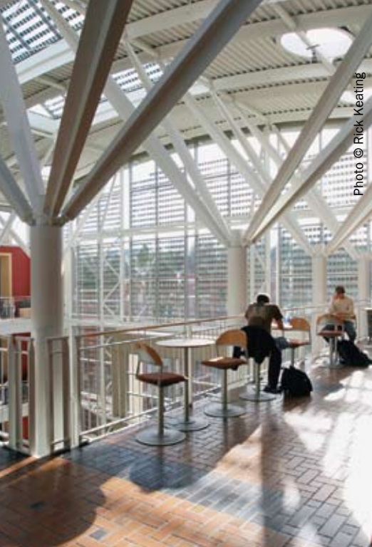
The atrium has no conditioned air supplied to it other than the recycled air from the classrooms.
